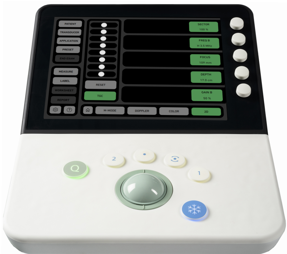
Figure 2-4. The control panel and touch screen.
